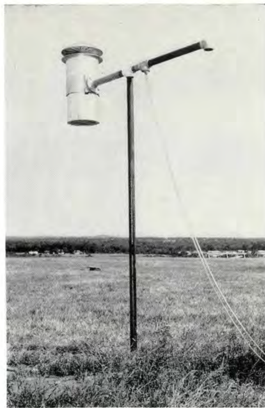
Left, transmissometer consists of a horizontal light projector and light sensitive receiver, installed 500 feet apart. Above, temperature-humidity set gives up-to-the-second indications on the runway complex. More accurate runway temperatures are expected.
